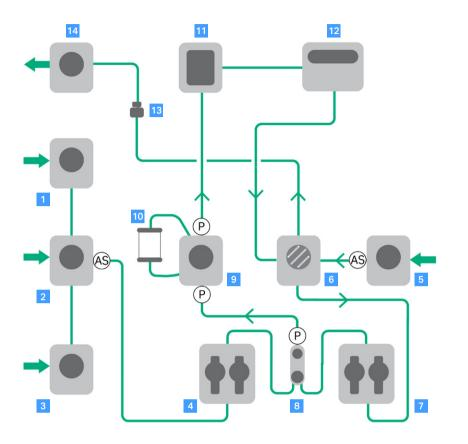
Amidite 1 valve Solvent A valve with air sensor Amidite 2 valve 4 System pump A Solvent B valve with air sensor 6 Recirculation valve System pump B 8 Pressure monitor 9 Column valve with pressure sensors Column Conductivity monitor UV monitor 13 Flow restrictor Waste valve
